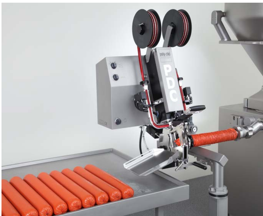
The PDC 700/800 closes all diameters up to 115 mm without any problems
